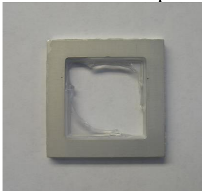
Figure 4. Initial frame with encapsulant “stuck” to it.
