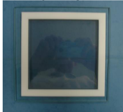
Figure 5. 125mm square Teflon containment frame on sticky surface on glass base plate.
