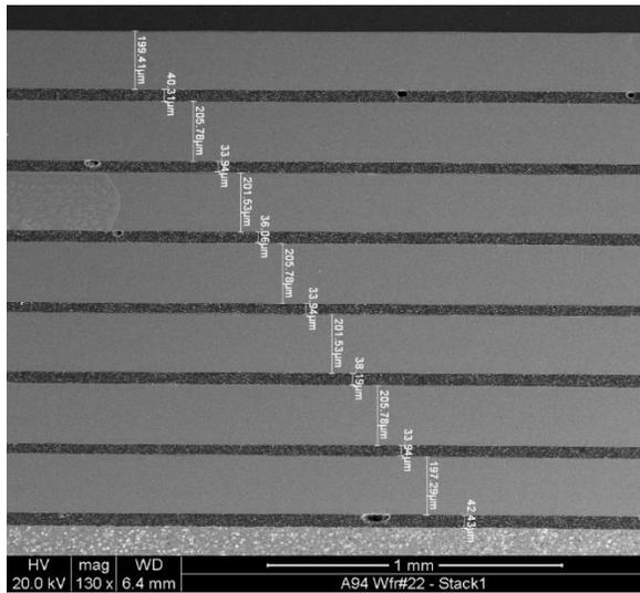
Fig 2. 7 die stack with high thermal conductive DAF.
