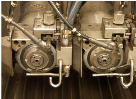
Fig 3 DDAF dicing on dual spindle saw
