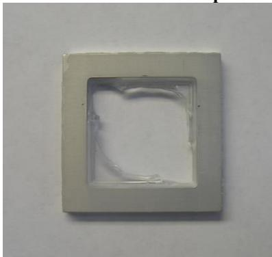
To eliminate that problem, the frame was fabricated from Teflon. This new frame, measuring ~125 mm square, and the placement fixture consisting of a sticky surface on a glass base, is shown in Figure 5 before any parts were placed or any encapsulant dispensed.
